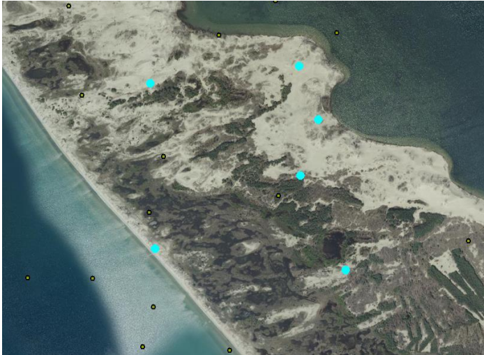
Figure 6. Steep slopes caused by sand dunes that result in large errors in elevation (The green points on the upper-right of the image showing greater errors) .
